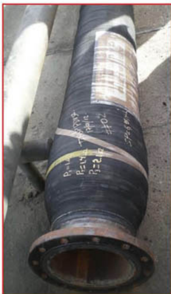
Hose with split outer vulcanised layer, and hose to replace it. (see test date on hose)
