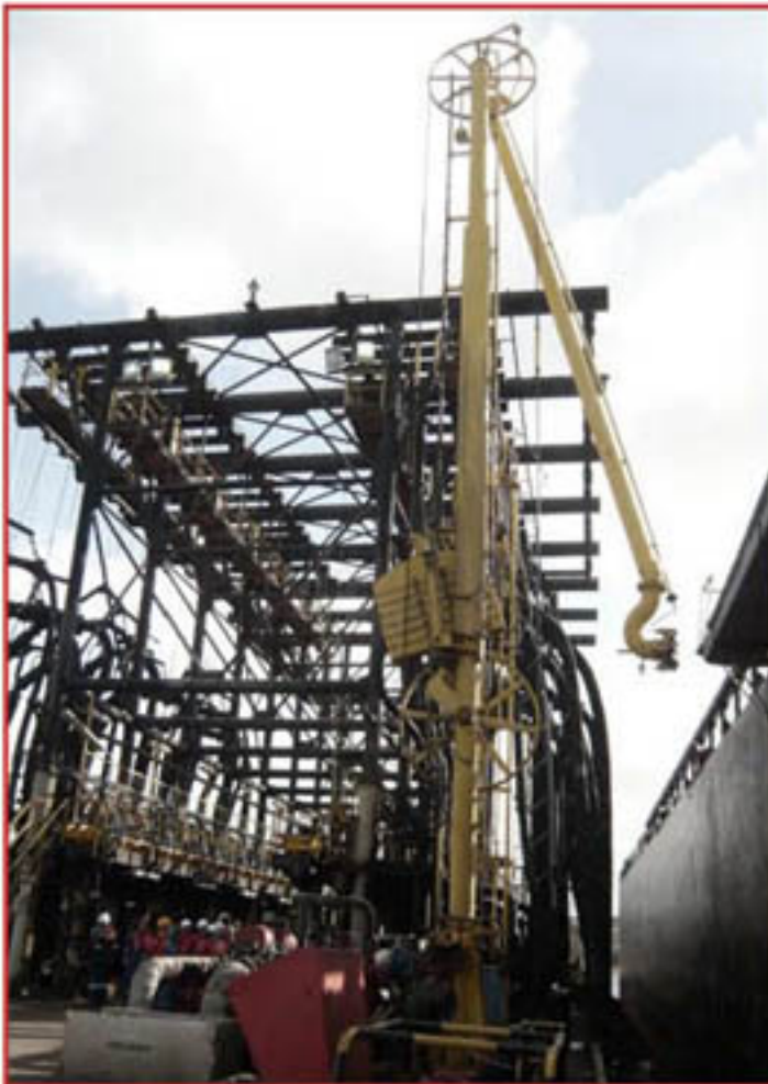
Mix of hoses for white products and articulated arms for LPG
